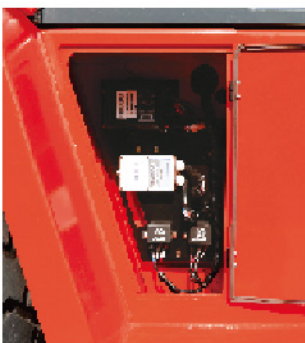
Sealed compartment for electrical controls
