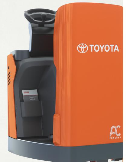
SIDESTANCE POSITION enables operators to easily change direction and travel long runs shuttling pallets from dock to stock or vice versa
