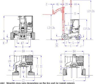
Note: The diagrams shown are for measurement reference and may not reflect the actual model. Weights may vary depending on the tire and /or torklitt options.
