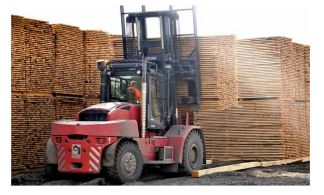
Designed specially for the lumber industry: a reversible cooling fan helps clear the cooler from harmful dust. The rotatable driver's seat lets the driver go "forward in reverse' with an unobstructed view even when fully loaded.
